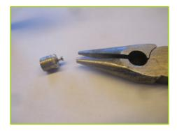
3. Using the needle nose pliers, pull the screw straight outward to remove the needle from where it is lodged.
